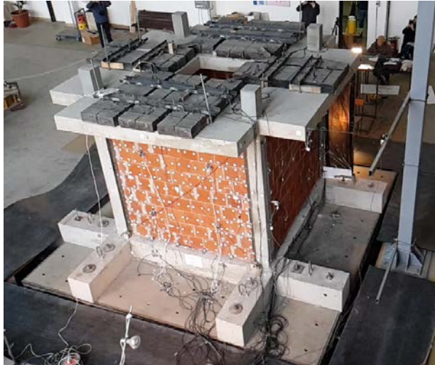
Figure 51: Completely instrumented and loaded test specimen placed on shake table
